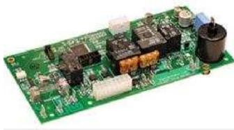
It's important to remember that although you may be operating your refrigerator in electrical mode or even LPG mode, the *control circuit* is powered by your 12VDC system. Therefore if you experience a problem with your 12VDC electrical or out dry camping and your 12VDC system voltage drops below 10.5VDC, your refrigerator control circuit can no longer function and the refrigerator will turn off.
